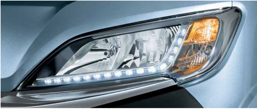
The LED DRL headlights (on request) are located in an area protected from impacts and guarantee 40% more light efficiency. They are available with a black or white frame to match the grille.
