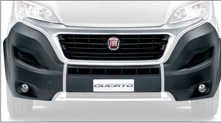
The new bumper comprises three components that can be removed individually, in addition to the grille, permitting rapid, cost-effective maintenance. Its shape ensures the utmost protection. The grille is available in metallic grey or “piano black” with “hot stamping”.
