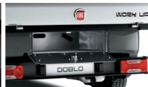
External compartment with lock for storing tools up to 2 metres in length
