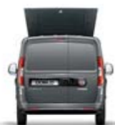
Rear roof window (opt. 585) available with 2-wing glazed or panelled rear door
