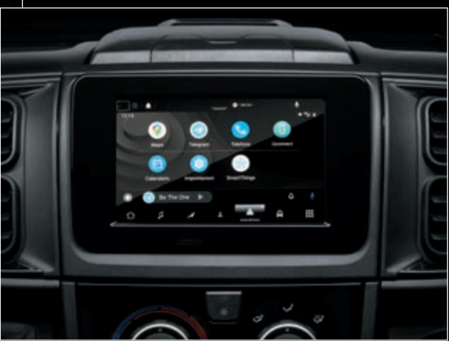
Uconnect™ 7" radio with 7" touchscreen color display, Android Operating System technology and steering wheel controls.
